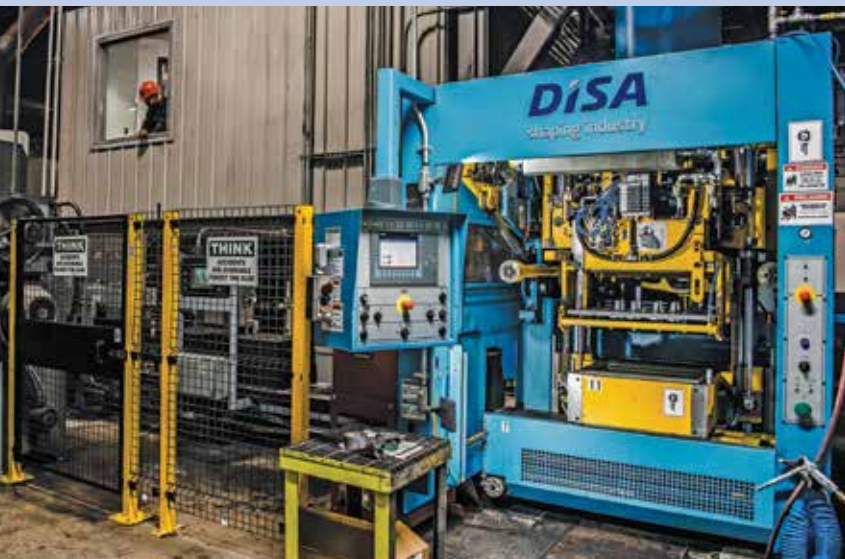
An employee watches the molding line for Buck’s new automatic molding machine that can produce up to 160 molds per hour. Buck also incorporated automatic pouring for perfect pours in each mold.
